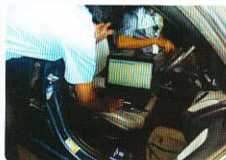
Mr.Suman - Team Leader conducting inspection of the vehicle through MDI.
