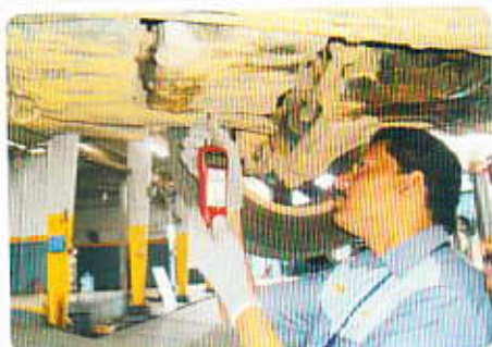
Mr.Noor Ahamad, Technician checking the Drive Belt tension.
